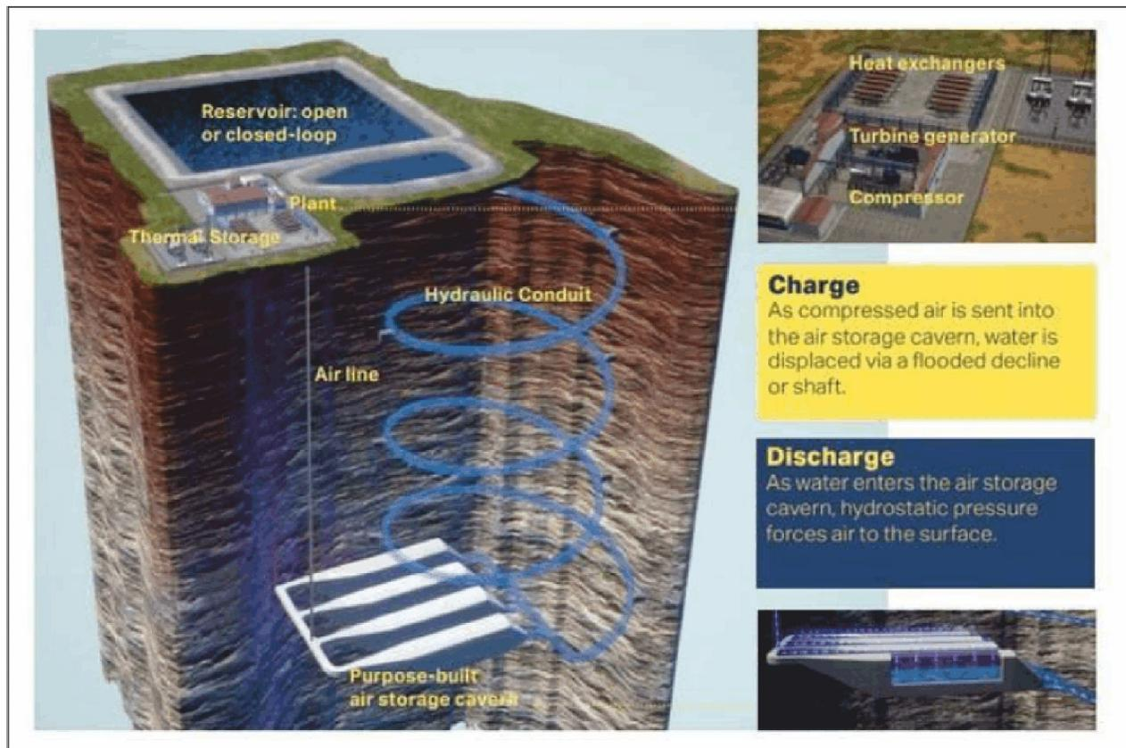
Unlike utilizing lithium-ion energy storage batteries, compressed air energy storage (CAES) is a way to store energy generated at one time for use at another time using compressed air. Basically, Hydrostor’s utility-scale storage systems pump large volumes of air into small underground shafts during off-peak hours and then releases it to run turbines when energy demand goes up.
